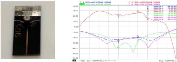
**Fig. 5 - Prototype of Ka-range Y-circulator and its electrical parameters**
