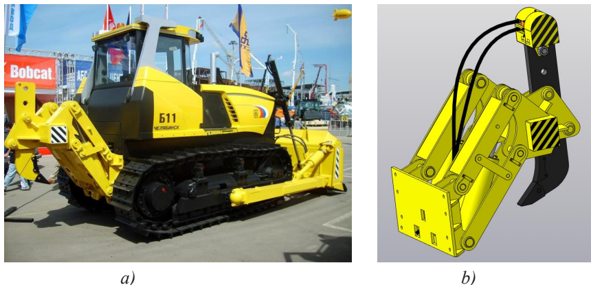
a) Figure 2 - Hinged vibration ripper of bulldozer-ripper B-11: a) bulldozer-ripper B-11 [8]; b) hinged vibration ripper
