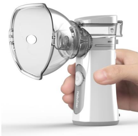
Fig. 5. Portable medical inhaler for children and adults. Power consumption 2 W, operating frequency of the piezoelectric nebulizer 110 kHz, container capacity 10 ml, atomization rate not less than 0.25 ml / min, droplet size not more than 3.7 microns, powered by AA batteries or via USB cable 5 B, 1 A
