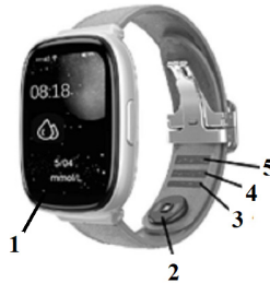
Figure 5. Wrist device for non-invasive monitoring of blood glucose and other parameters of the human body by blood.
