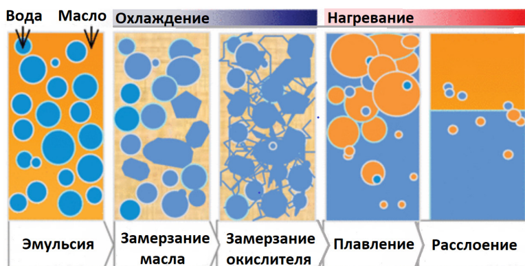
Figure 1. Destruction of the inverse emulsion during the “freeze-thaw” processes [9].
