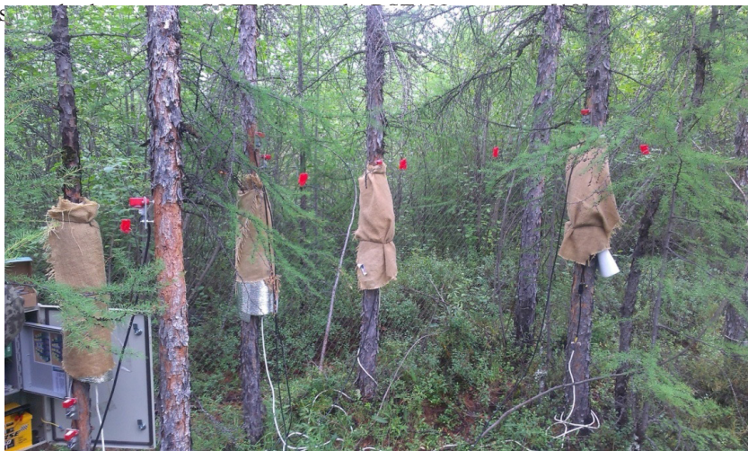
Fig. 1. Experimental Gmelin larch trees in a cryogenic larch forest with DRL-26 belt dendrometers installed on them.
